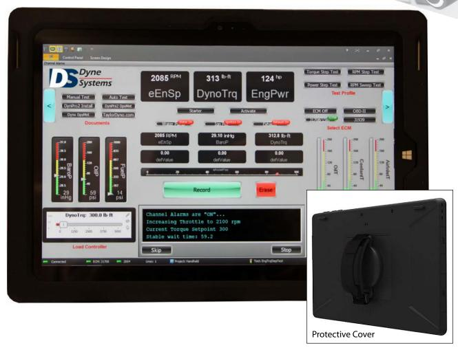
The Surface Pro Tablet accessory allows the operator complete control away from the test cell and/or testing equipment yet still provides access to the data acquisition and control system. This is a great capability to have for system calibration, troubleshooting and more.
