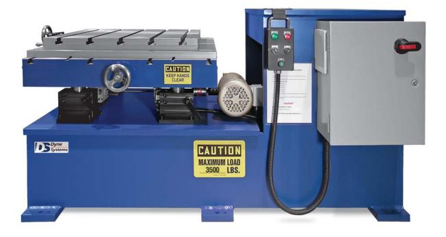
The XYZ Lift Table Test Stand allows the testing of electrical motors with varied horizontal or vertical center lines. It features a fixture mounting plate that can be adjusted on the X-Y-Z axes. The X and Z axes are controlled through manual crank handles while the Y axis is adjusted through a remote pendent which controls a powered AC gear motor with mechanical actuator.
